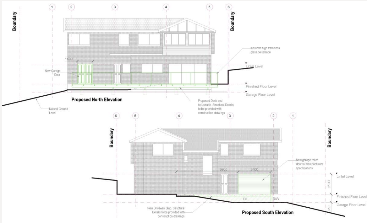
Figure 11 – Proposed north and south elevation.
